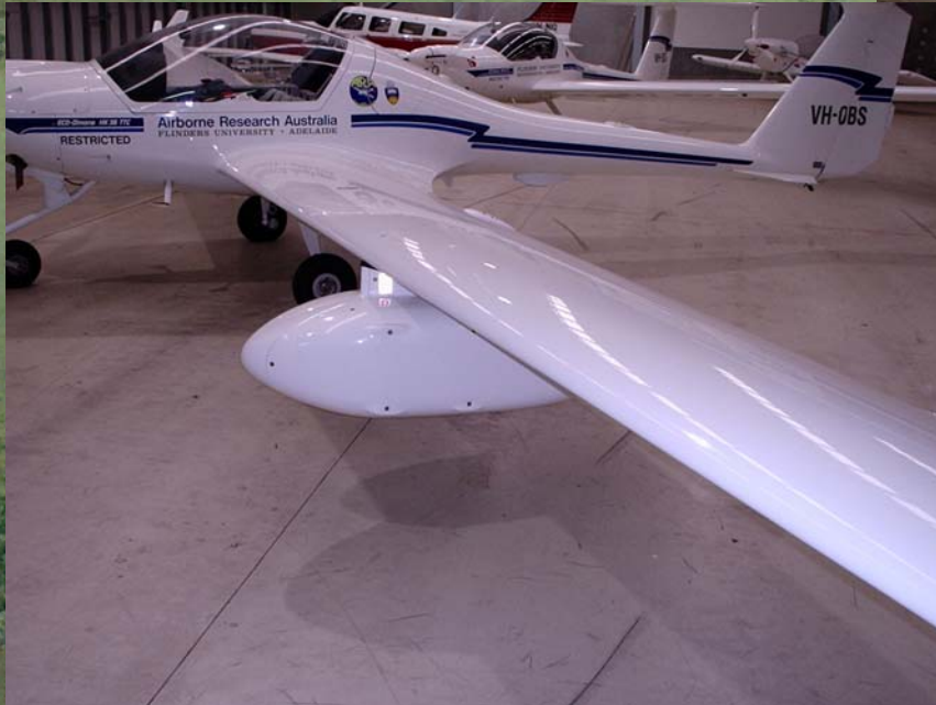
The Remote Sensing Pod installed under the wing of the ARA ECO-Dimona
