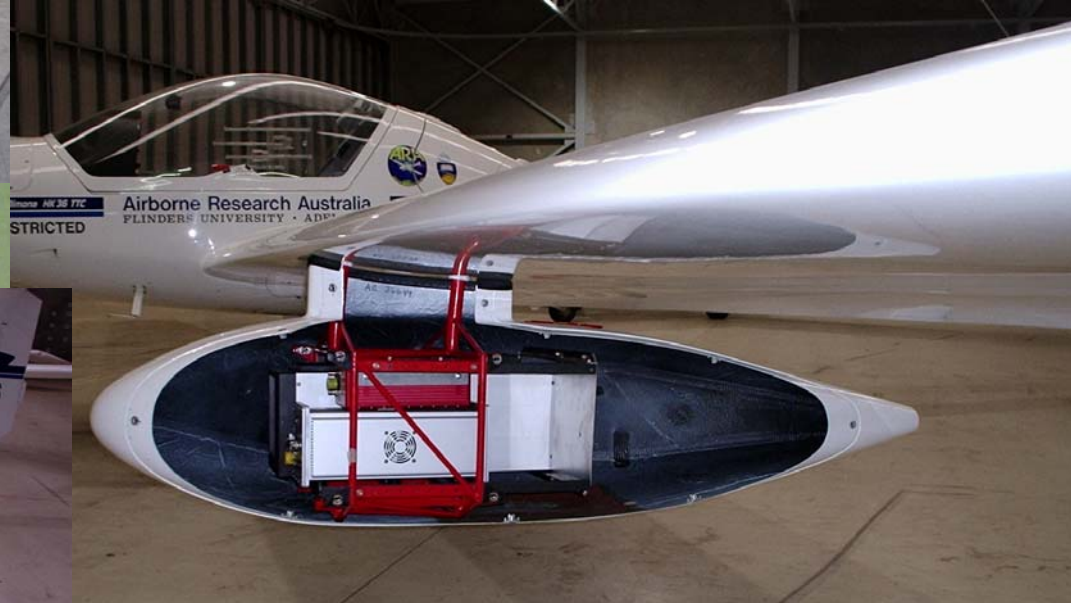
The Remote Sensing Pod installed under the wing of the ARA ECO-Dimona
