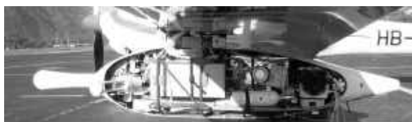
Figure 2: Left instrument pod with 5-hole gust probe with integrated pressure sensors in the nose-boom. Just behind the boom, the IRGA is visible, then the CO-monitor and the NO x TOy with external peristaltic pump and NO y -converter at the rear. All the rest listed in table 1 is in between.
