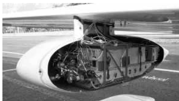
Figure 3: Right instrument pod with gas chromatography system including pressurized gas for operation (H 2 as carrier gas, CO 2 to cool the cryo-trap). Behind: The LICOR as redundant CO 2 /H 2 O-instrument (closed system, with intake away from CO 2 -exhaust of GC). Construction detail: The steel frame in the pod is supporting all installations; also the rest of the cover can be removed in a minute. On top, cabling and tubing is entering a 2" flexible aluminum tube which leads via the wing into the fuselage.
