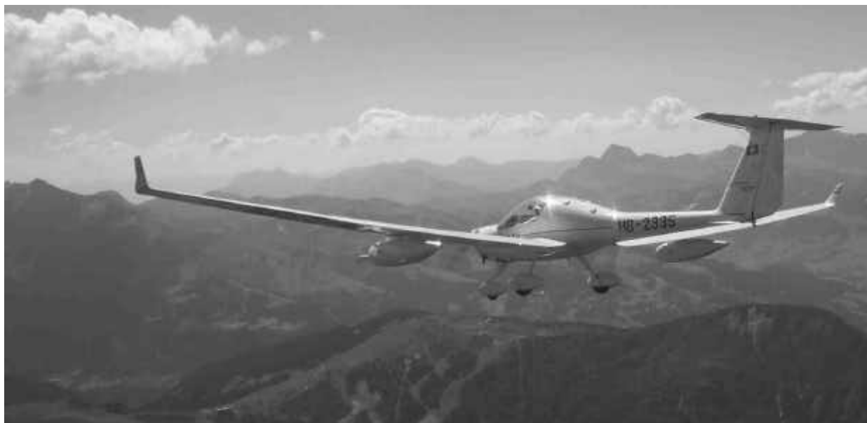
Figure 1: MetAir's 'Dimona' during a mission in the Swiss Alps, Summer 2000 (Foto Joerg M. Hacker). Each underwing pod is containing up to 50 kg of instrumentation (fig. 2 and 3, table 1). Details about the aircraft in table 2.
